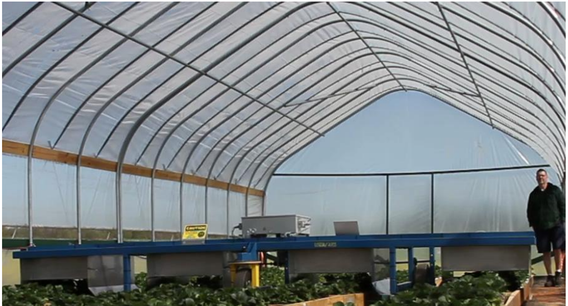
Supplementary Figure S1. Self-propelled UV-C irradiation apparatus with four irradiation units covering four raised beds with strawberry plants in high tunnel at the USDA-ARS Appalachian Fruit Research Station in Kearneysville, WV.
