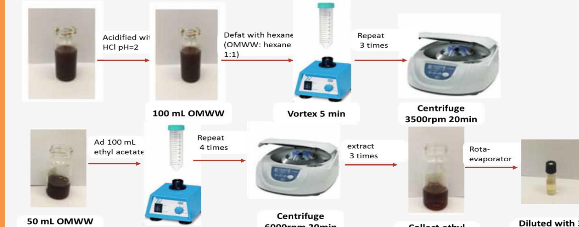
Fig 2. extraction procedure of phenolic compounds from OMWW
